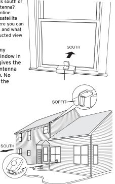
you receive a consistent signal, or placing the antenna in a window is not a practical solution for you, **BETTER** reception can be achieved by placing the antenna outside on a window ledge, porch, table, or patio. The location you choose should provide the antenna with a clear view of the southern sky.
