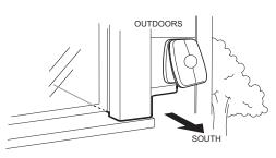
To mount the antenna, you will need four screws (not included) with a 1/4" head (e.g., an M3 screw), and that are suitable for the material onto which you are affixing the antenna, (e.g., wood, metal, etc.). The screws should be spaced 30 mm (1-3/16") apart horizontally and 36.5 mm (1-7/16") vertically. Refer to the template on "Indoor/Outdoor Antenna Template" on page 44.
