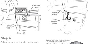
to install, route and hide the antenna cable and the FMTA cable. Be sure to coil and secure any excess cable in a hidden location, such as under the carpet on the passenger side, keeping it away from vehicle pedals and controls. The bundled cables should be as far away from the CLA power cable as possible (see *Figure 20*).
