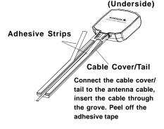
Remove the remaining protective tape from the adhesive, carefully position the antenna with cover/tail and apply pressure to secure to the vehicle.
