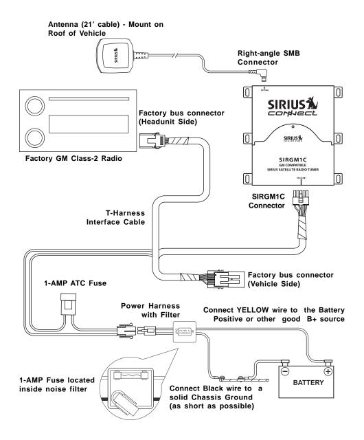
NOTE: If your vehicle is equipped with a factory satellite radio tuner and you are using the included 'T-harness interface cable' for installation, you must disconnect the factory satellite radio tuner at the tuner box. Otherwise, operational errors will occur while using the SIRGM1C.
