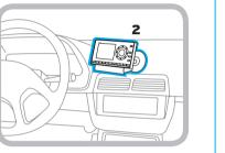
B. Orient the adhesive foot so that your Radio is easily accessible. Loosen the knob and adjust the adhesive foot to position 1 or 2, and then tighten it.
